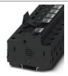
Fuse modular terminal block, Connection method: Screw connection, Cross section: 1.5 mm²- 25 mm², AWG: 16 - 4, Nominal current: 32 A, Nominal voltage: 600 V, Width: 18 mm, Fuse type: Class CC, Fuse type: Glass, Mounting type: NS 35/7,5, NS 35/15, Color: black
