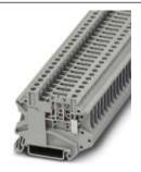
Disconnect terminal block, With test socket screws for insertion of test plugs, Connection type: Screw connection, Cross section: 0.14 mm<sup>2</sup> - 6 mm<sup>2</sup>, AWG: 26 - 10, Nominal current: 20 A, Nominal voltage: 500 V, Length: 57.8 mm, Width: 6.2 mm, Color: gray, Assembly: NS 35/7,5, NS 35/15
