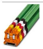
Feed-through terminal block, Connection method: Screw connection, Cross section: 0.2 mm<sup>2</sup> - 10 mm<sup>2</sup>, AWG: 24 - 8, Width: 8.2 mm, Color: white, Mounting type: NS 35/7,5, NS 35/15
