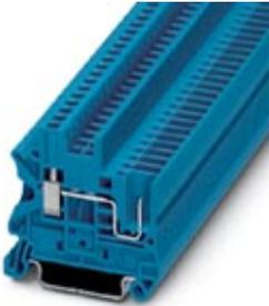
Feed-through terminal block, Connection method: Screw/plug-in connection, Cross section: 0.14 mm<sup>2</sup> - 4 mm<sup>2</sup>, AWG: 26 - 12, Width: 5.2 mm, Color: blue, Mounting type: NS 35/7,5, NS 35/15
