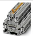
Knife disconnect terminal block, connection method: Screw connection, cross section: 0.14 mm² - 6 mm², AWG: 26 - 10, width: 6.2 mm, color: gray, mounting type: NS 35/7,5, NS 35/15
