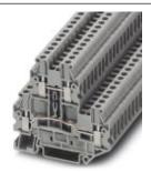
Double-level terminal block, Connection method: Screw connection, Cross section: 0.14 mm<sup>2</sup> - 4 mm<sup>2</sup>, AWG: 26 - 12, Width: 5.2 mm, Color: white, Mounting type: NS 35/7,5, NS 35/15
