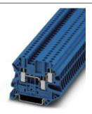
Feed-through terminal block, nom. voltage: 500 V, nominal current: 24 A, connection method: Screw connection, number of connections: 3, cross section:0.14 mm² - 4 mm², AWG: 26 - 12, width: 5.2 mm, height: 46.9 mm, color: blue, mounting type: NS 35/7,5, NS 35/15
