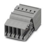
COMBI receptacle, Connection method: Plug connection, Number of positions: 4, Cross section: 0.08 mm² - 4 mm², AWG: 28 - 12, Width: 20.8 mm, Height: 18.8 mm, Color: gray
