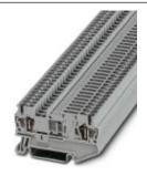
Disconnect terminal block, Connection type: Spring-cage connection, Cross section: 0.08 mm<sup>2</sup> - 4 mm<sup>2</sup>, AWG: 28 - 12, Nominal current: 20 A, Nominal voltage: 400 V, Length: 60.5 mm, Width: 5.2 mm, Color: gray, Assembly: NS 35/7,5, NS 35/15
