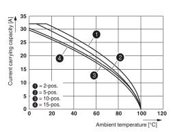
The figure shows the derating curve of the ST 4... terminal block in connection with the SP 4 plug
