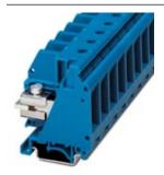
N disconnect terminal block, Special and hybrid connection, Cross section: 0.75 mm² - 50 mm², AWG: 18 - 1/0, Width: 15.2 mm, Color: blue, Mounting type: NS 35/7,5, NS 35/15, NS 32
