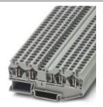
Feed-through terminal block, Connection method: Spring-cage connection, Cross section: 0.08 mm² - 6 mm², AWG: 28 - 10, Width: 6.2 mm, Color: blue, Mounting type: NS 35/7,5, NS 35/15
