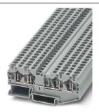
Feed-through terminal block, nom. voltage: 800 V, nominal current: 32 A, connection method: Spring-cage connection, number of connections: 4, cross section: 0.08 mm² - 6 mm², AWG: 28 - 10, width: 6.2 mm, color: gray, mounting type: NS 35/7,5, NS 35/15
