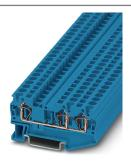
Feed-through terminal block, nom. voltage: 800 V, nominal current: 32 A, connection method: Spring-cage connection, number of connections: 3, cross section: 0.08 mm² - 6 mm², AWG: 28 - 10, width: 6.2 mm, color: blue, mounting type: NS 35/7,5, NS 35/15
