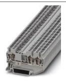
Feed-through terminal block, Connection method: Spring-cage connection, Cross section: 0.08 mm<sup>2</sup> - 1.5 mm<sup>2</sup>, AWG: 28 - 16, Width: 4.2 mm, Color: blue, Mounting type: NS 35/7,5, NS 35/15
