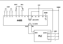
Note: The Reset & Hold switches shown in the above wiring diagrams are optional and are not required for all applications.
