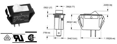
Mounting Hole: 0.55" x 1.125" \_\_\_\_\_
