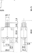
Specifications: Standard Rating: 3-20 AMPERE. Input Power: 125 VAC / 250 VAC Dielectric Strength: 1500 VAC / 1 Minute.
