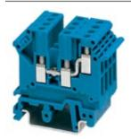
1-level terminal block with double connection on one side, cross section: 0.2 - 2.5 mm², AWG: 30 - 12, width: 5.2 mm, color: blue
