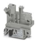
Feed-through terminal block, mounting type: NS 35/7,5, NS 35/15, NS 32, number of positions: 1, pitch: 5.08 mm, width: 5.08, color: gray
