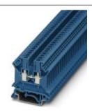
Feed-through terminal block, Connection method: Screw connection, Cross section: 0.2 mm² - 4 mm², AWG: 24 - 12, Width: 5.2 mm, Color: blue, Mounting type: NS 32, NS 35/15, NS 35/7,5
