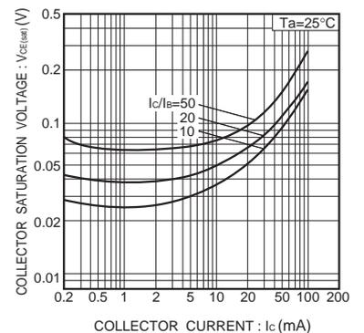
Fig. 6 Collector-emitter saturation voltage vs. collector current
