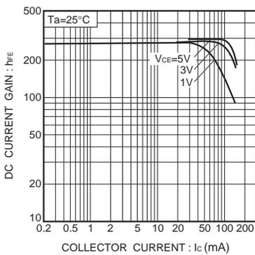
Fig.4 DC current gain vs. collector current ( I )
