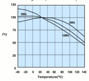
Measured on a 2644000301 using the HP4291A.
