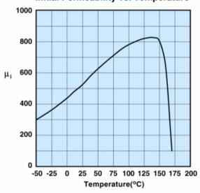
Measured on a 17/10/6mm toroid at 100kHz.
