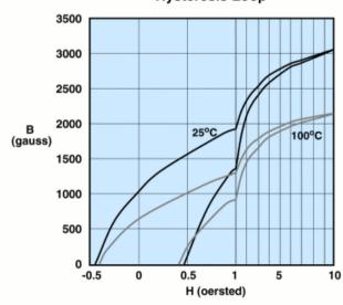
Measured on a 17/10/6mm toroid at 10kHz.
