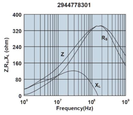
Impedance, reactance, and resistance vs. frequency.
