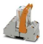
Pre-assembled relay module with push-in connection, consisting of: relay base, power contact relay, and retaining bracket. Contact type: 3 PDTs. Input voltage: 24 V DC
