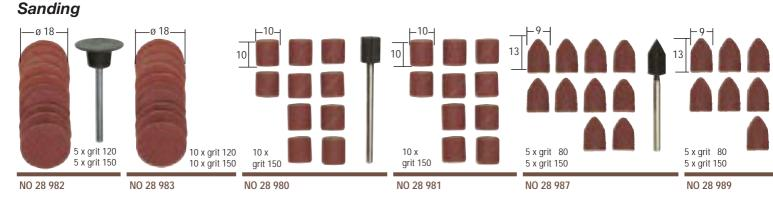
Sanding discs, drums and wheels Made of standard compounds of tough consistency and different grits for different sanding stages. With superior lasting characteristics and of various shapes for numerous operations. All shafts 3.0mm. For working steel, non-ferrous metals, plastic, rubber, leather, wood (even edges). Rough grinding of V2A-steel, grinding, welding joints and die-cast aluminium. Ideal for surface and shape sanding.
