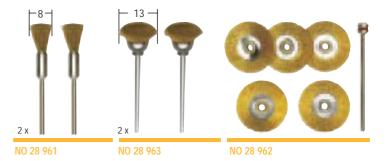
Brass brushes, cups and wheels Ideal for working on alloys, copper, precious metals, semi-precious stones, plastic and wood. Acid proof. Electrically neutral, thus suitable for working with electronic components.
