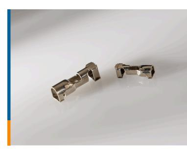
TE Connectivity (TE) introduces the Slim Wire to Board Connector that was developed for wire to PCB board connection. The slim connector with no housing serves as an easy poke in connector with strong retention ability. The advantage of using this connector is that the conductor can be connected quickly without special tools and the small profile saves the space on the PCB.
