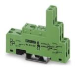
PR1... relay base, for miniature power relays or miniature switching relays with 1 or 2 changeover contacts or solid-state relays of the same design, 1/3-level version, screw connections, plug-in option for input/interference suppression modules
