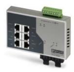
Ethernet Switch, 6 TP RJ45 ports, 2 FO ports, 100 Mbps full duplex in SC-D format, automatic detection of data transmission speed of 10 or 100 Mbps (RJ45), autocrossing function
