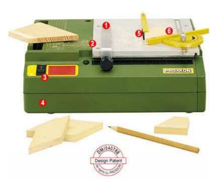
The 58mm diameter super-cut blade cuts soft woods up to 8mm. The 85W VDE tested motor is quiet, operates off 220 - 240V and has a prolonged life expectancy. Cutting performance: in wood up to 8mm, plastics (Pertinax too) to approx. 3mm, non-ferrous metals to approx. 1.5mm. Even fibreglass reinforced PC cards can be cut with the tungsten blade. The side door allows easy sawdust removal. Overall size approx. 240 x 180 x 80mm. Weight approx. 1.8kg.
