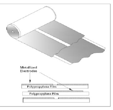
Regal-Beloit's GEM III capacitors are manufactured with high-grade metallized polypropylene film. This film is in the range of 5 to 10 microns thick, depending on the application, voltage, and conditions. The metallized electrode is several hundred angstroms thick.
