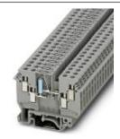
1-level terminal block with double connection on both sides, with fitted resistor 499  $\Omega$ , ± 0.1%, 0.5 W, TCR ± 10 ppm/K, cross section: 0.2 - 2.5 mm<sup>2</sup>, width: 6.2 mm, color: Gray
