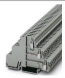
Sensor/actuator terminal block, Cross section: 0.2 mm² - 4 mm², AWG: 24 - 12, Connection type: Screw connection, Width: 6.2 mm, Color: gray, Mounting type: NS 35/7,5, NS 35/15
