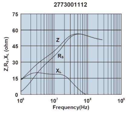
Impedance, reactance, and resistance vs. frequency.
