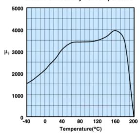
Measured on a 17/10/6mm toroid at 10kHz.
