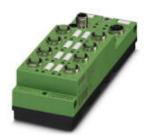
The stand-alone device for PROFIBUS has 8 digital inputs. The M12 connection is established using fast connection technology. The 24 V DC supply is protected against short circuit and overload. The nominal current of the device is 600 mA.
