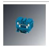
1-level terminal block with double connection on both sides, cross section: 0.2 - 2.5 mm², AWG: 30 - 12, width: 5.2 mm, color: blue
