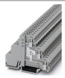
Sensor/actuator terminal block, With equipotential bonder, connection method: Screw connection, cross section: 0.2 mm² - 4 mm², AWG: 24 - 12, width: 6.2 mm, color: gray, mounting type: NS 35/7,5, NS 35/15
