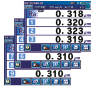
Trace display: the ten latest measurement results using the same parameter
