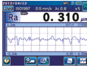
Profile display: one parameter measurement result and the measured profile
