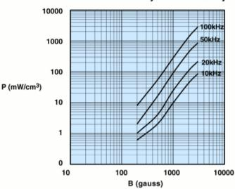
Measured on a 17/10/6mm toroid using the Clarke Hess 258 VAW at 100°C.
