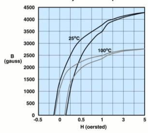
Measured on a 17/10/6mm toroid at 10kHz.
