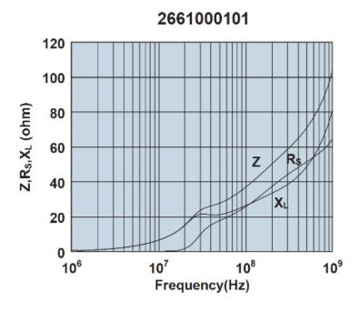
Impedance, reactance, and resistance vs. frequency.
