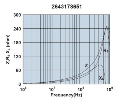
Impedance, reactance, and resistance vs. frequency.
