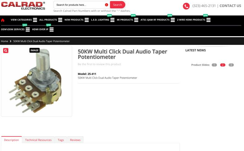
**25-411 | MINIATURE MULTI-CLICK DUAL CONTROL- 40 STEP P.C. MOUNT** 11/16" dia., 11/4" long overall, 9/32" hole size, 1/4" dia shaft, 9/16" long shaft including threads.1/4 watt, 20% tolerance, 300° rotation. Solderable terminals.
