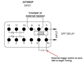
†If the jumper wire shown in each diagram is replaced by a resistor, delay time will be added to that which is produced by an internal fixed resistor on fixed time models (Code F) or any setting on screwdriver adjustable models.
