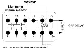
DOUBLE POLE DOUBLE THROW WITH NORMALLY OPEN CONTACT DOUBLE POLE DOUBLE THROW
