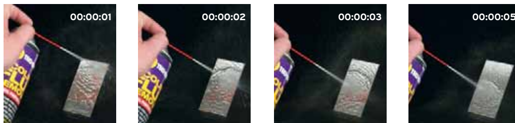
G3 and Ecoline defluxers easily clean tough baked-on rosin flux contaminants in 3-5 seconds.
