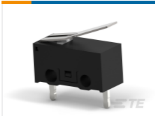
TE Model / Part # 2351447-5 UMINSA SW BLV0.88N 3A /1.5A AC NC PCB
