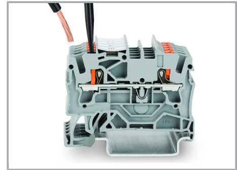
Insert fine-stranded conductors via operating tool.
