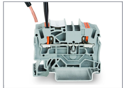
Insert fine-stranded conductors via operating tool.
