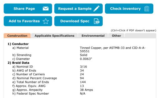
Alpha braid is an exceptional, low resistance way to create a point-to-point ground strap. In retrofit applications, braid is an ideal way to install additional shielding to your cable.
