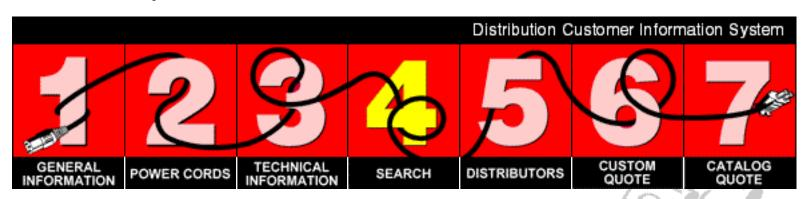
Back **Selected Cable: 2136H Cord View** End View Cord Plug Connector **End View** C-19 C-20 **SJT** n/a 2136H Part Number 3 conductor plastic detachable Category hielding unshielded **Jacket Color** Black 8.2 Ft Length Feet **Length Meters** 2.5 meters **Temperature Rating** 105 C°C Packaging Units Per Carton 25 Approvals 14 AWG Stranding .380 **Nominal OD Inch** 16A-250V Rating
