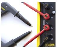
\* For Models 6240 and 6255 instruments with serial numbers lower than 116339SEDV, terminals C1 and P1 are red, and C2 and P2 are black. In this case, connect probes as shown in the table on the following page.
