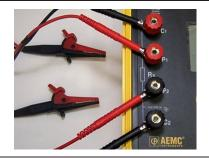
For the probes with Red/Blk and Red/Blk leads and Red DOT located on the probe tip: Connect them as shown here.
